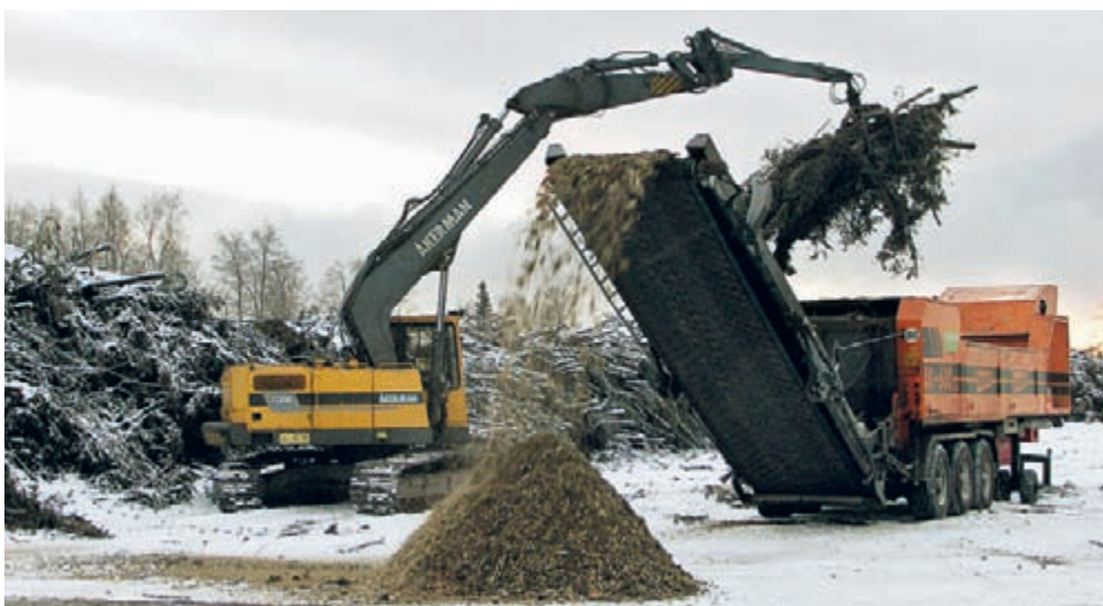
Manufacturing biofuel from untrimmed tops and branches at one of Billerud's mills.
